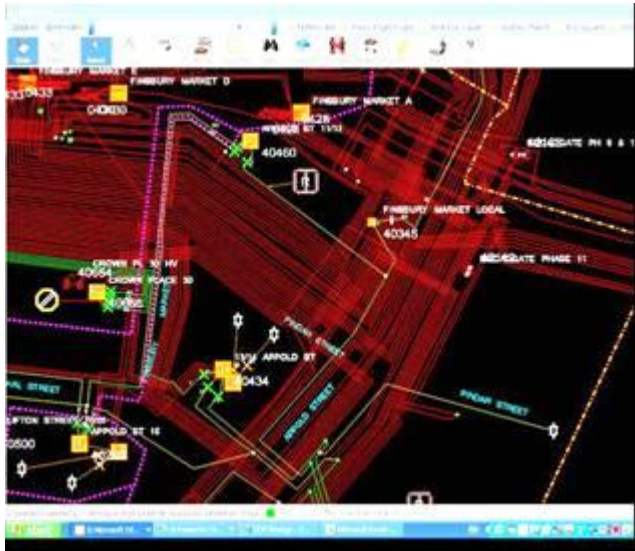
Figure 21: The mass of 60 HV cables (red lines) in the vicinity of the fault outside Finsbury market primary substation
