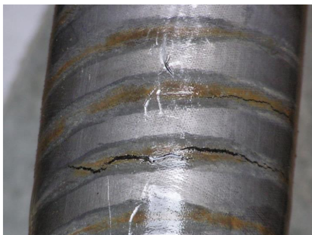
Figure 16 – Crystallised lead sheath
