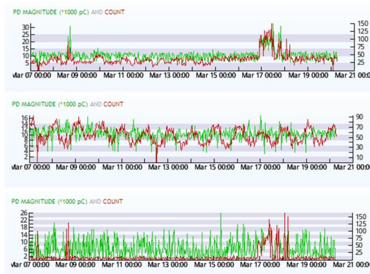
Figure 27– Partial discharge activity of 11kV cables at Brighton Town substation (SPN)
