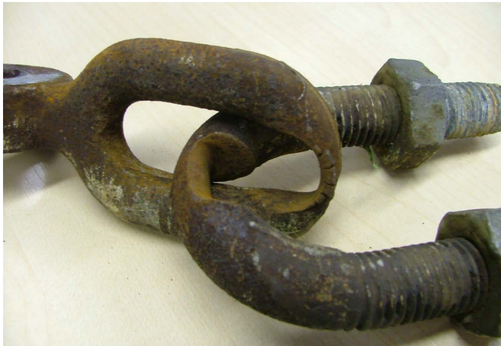
Figure 10 : A worn shackle showing the extent of degradation that can occur on fittings from mechanical processes such as wear
