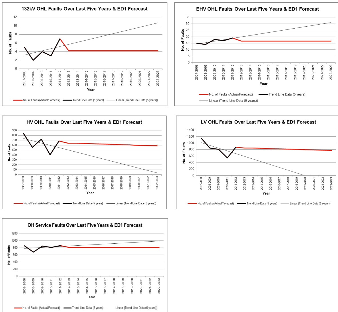
Figure 51 Overhead Line Fault Trends (Data Source: Fault Analysis Cube)
