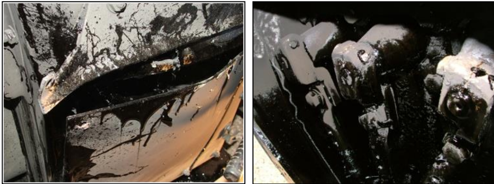
Figure 17: Serious Compound Leak
