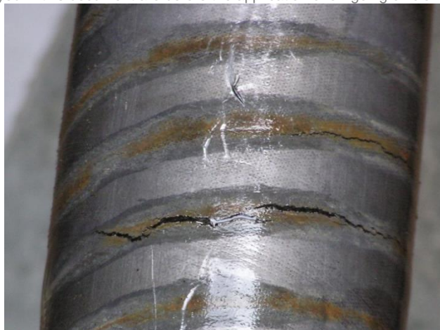
Figure 20 – Crystallised lead sheath
