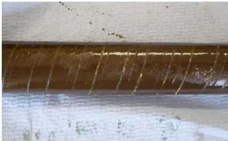
Figure 9: Minor waxing on inner insulation papers
