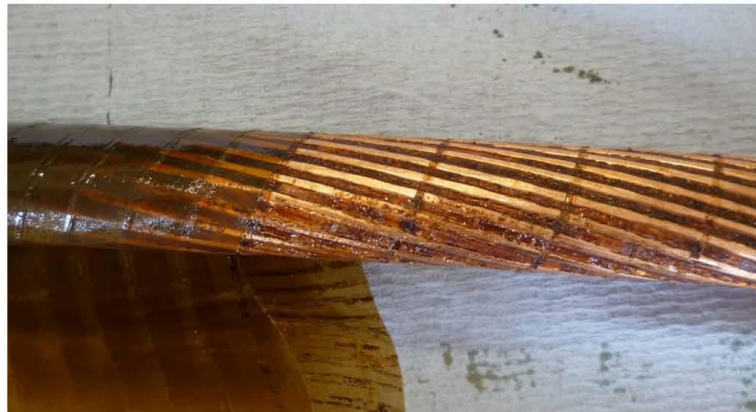
Figure 10 Hardened cable compound on strands
