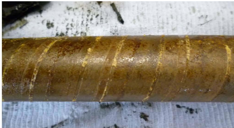
Figure 5 Wax at butt gaps
