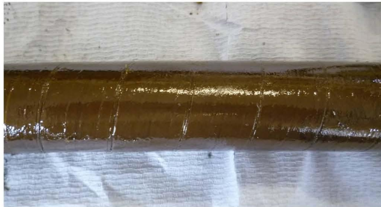
Figure 8: Oily outer insulation papers
