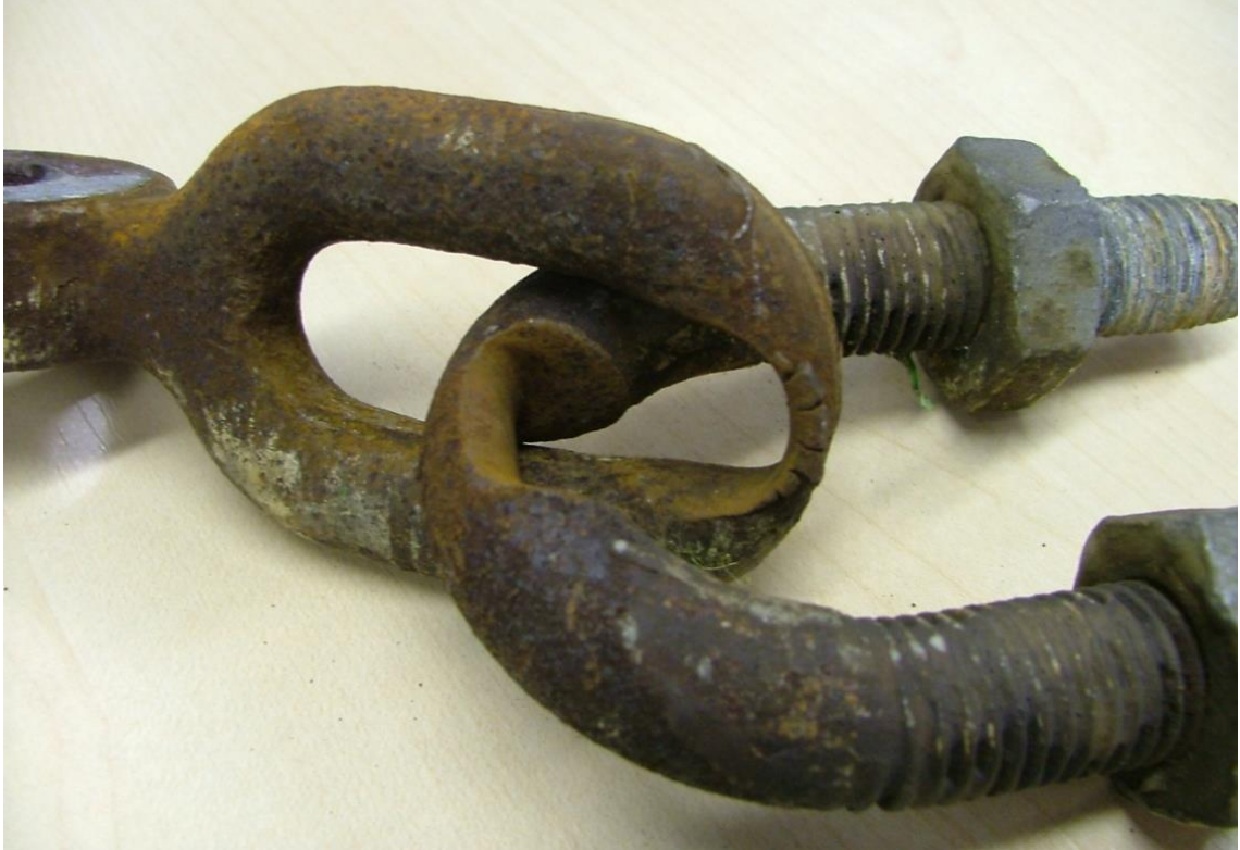
Figure 8 : Photo of a worn shackle, showing the extent of degradation that can occur on fittings from mechanical processes such as wear
