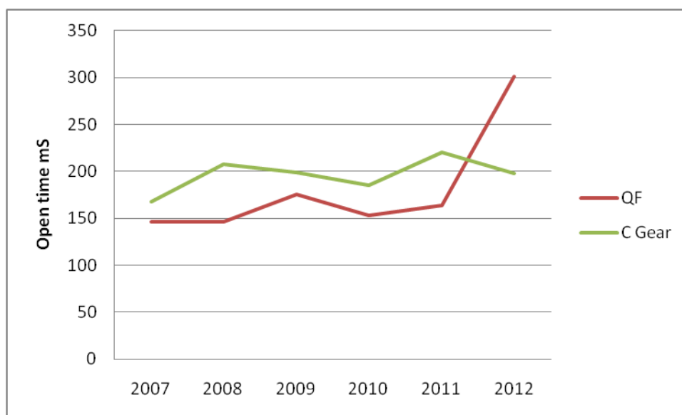
Figure 10 – CB trip times for Reyrolle 'C' and AEI 'QF' from Enmac control system
