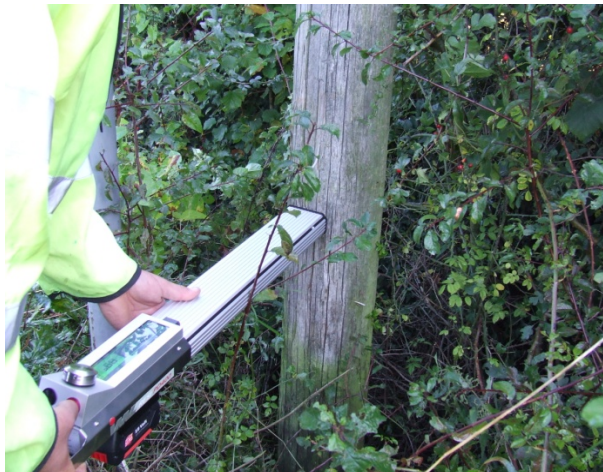
Figure 31 – Micro-bore pressure sensing drill in use and output information
