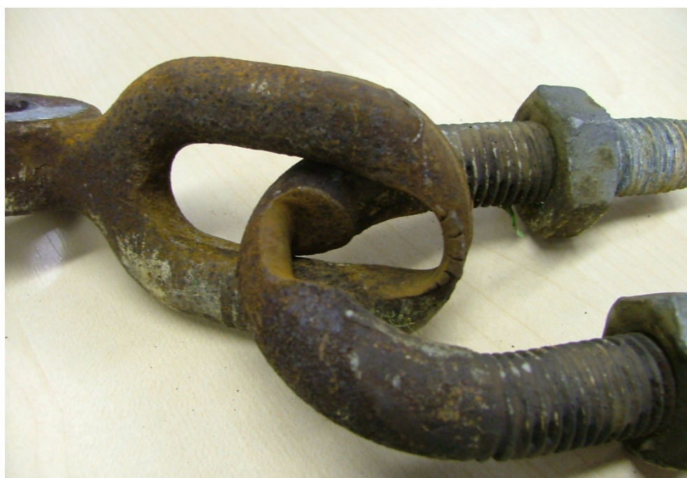
Figure 12: Photo of a worn shackle showing the extent of degradation that can occur on fittings from mechanical processes such as wear
