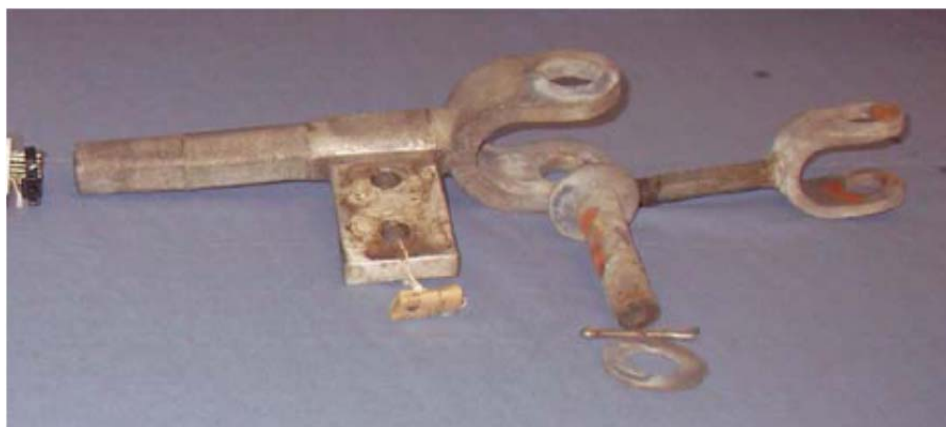
Figure 3 - Failed Compression Fitting
