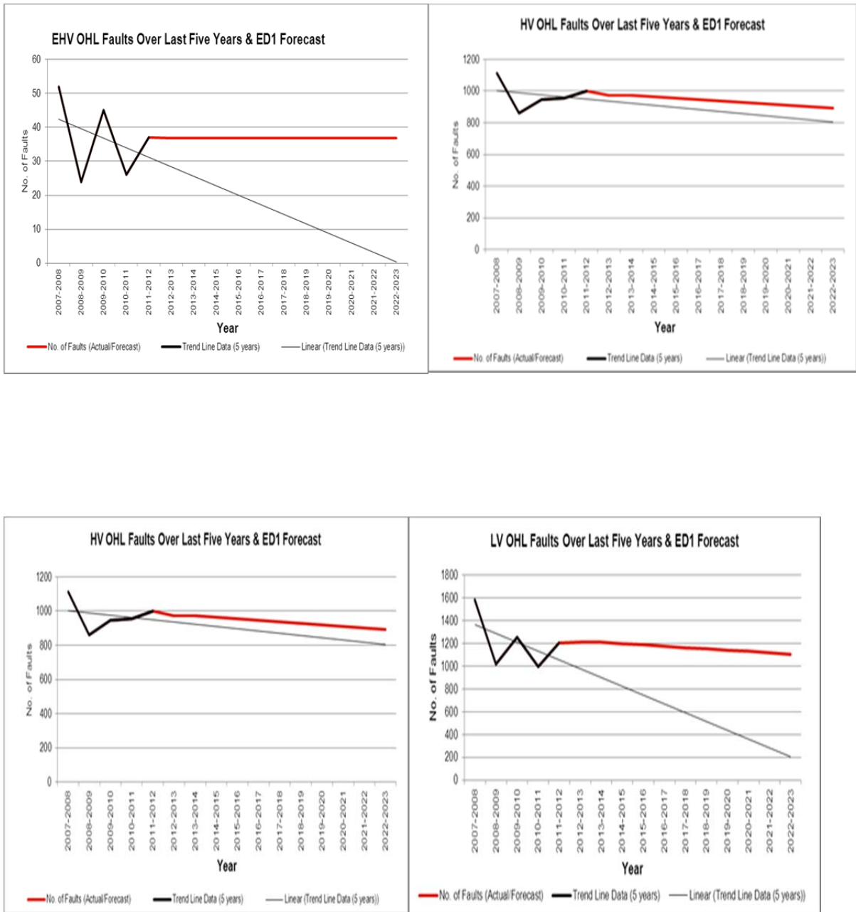
Figure 49 Fault trends for wood pole overhead lines
