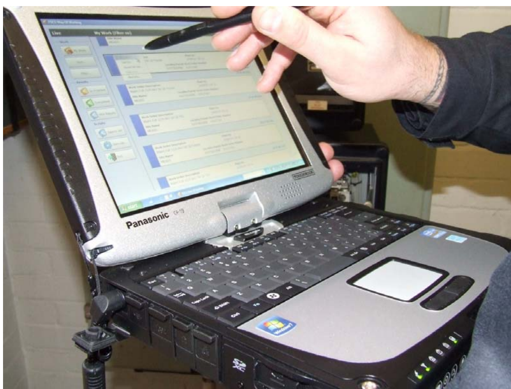
Figure 45- Recording equipment condition on a portable device for automatic updating of the asset register
