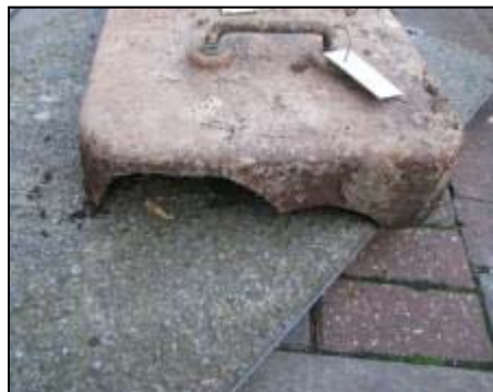
Figure 21: Broken Bell Cover
