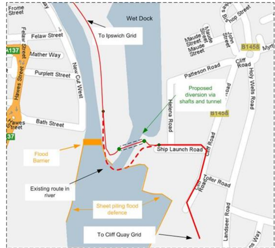
Wet Dock 132kV diversion
